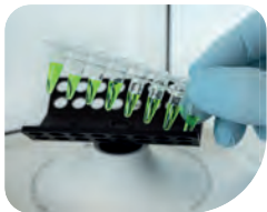
PCR Strip Rotor holds two, 0.2 ml 8-strips or 32 x 0.2 ml single tubes.
